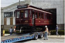
As you read in column 1, the lowboy trailer was equipped for this job but the real surprise was when we arrived and the car was to be unloaded. The car would actually be unloaded from the front of the trailer. Very carefully the trailer brakes are set and the tractor is detached, with the skill of the truck driver being responsible for gently lowering the trailer to the ground.
