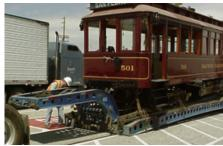
In what we found fascinating, the gooseneck portion of the trailer, shown in the above photo just in front of car 501 would be detached by removing the front two attaching points and backing the tractor back under the gooseneck, removing the rear attachment and pulling away.
