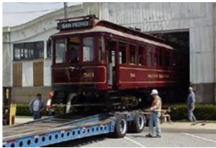
The car was moved with the hand brakes applied. This was done to eliminate any possibility of a runaway.
